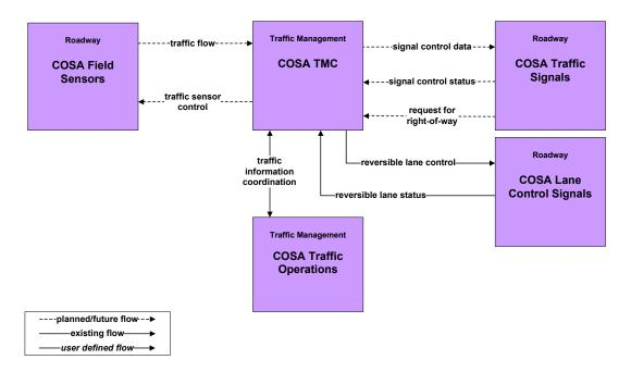
Figure 5 – Example Market Package Diagram: Surface Street Control
